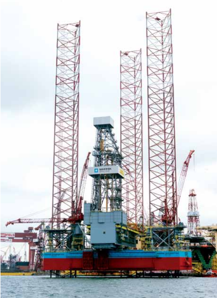
Keppel FELS delivered one of the world's largest jackup rig, XLE-2, to Maersk Drilling on budget and seven days ahead of schedule. It is the second of three XLE rigs that Keppel is building for Maersk
